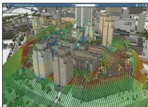
Photo 12: 3D Wind flow analysis of a Singapore development
