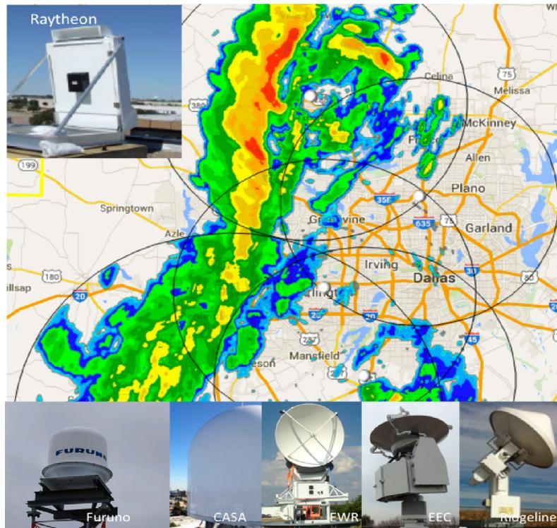
Figure 10. Urban radar network. Networks of small radars (bottom images; black circles show location and range in top image) are deployed in the Dallas–Fort Worth area to solve the Earth curvature low-level detection problem. These radars are expected to be replaced by low-cost, low-maintenance, low-infrastructure X-band phased arrays radars (upper left and lower left image).
